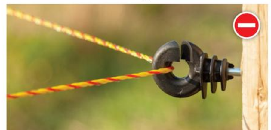
Do not use ring insulators at the corners
