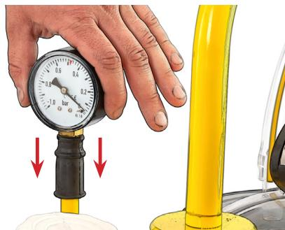
Connect the bucket and the machine. On the bucket lid, attach the tube to the inlet with the milk stopper.
