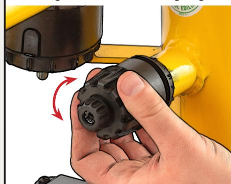
After completing the adjustment, tighten the locking nut firmly without letting the regulator body shift.
