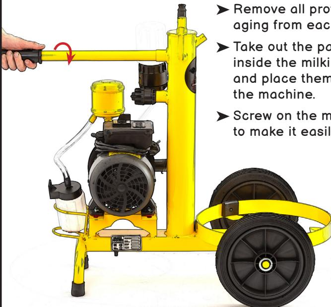
It is recommended to perform the assembly at a temperature above 20 °C to make it easier to fit the hoses. If the hoses are difficult to attach, moisten their interiors with water or gently warm the ends with a heat gun.
