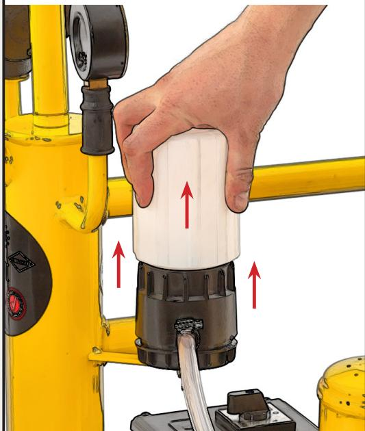
Screw back the cap back onto the container.
